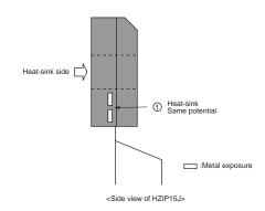
• Frame diagram (LV5693P) \*In the system power supply other than LV5693P, pin assignment may differ.
