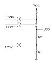
The FB voltage is determined by the internal band gap voltage of the IC (typ = 1.26V)
